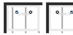
Where joists run parallel to the width of the tray, at least one hole will always be clear.
