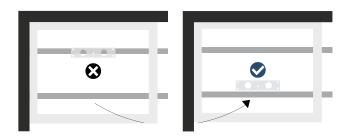
Where joists run parallel to the length of the tray and both holes are obstructed, simply turn the tray  $180^{\circ}$ . The unique offset position will ensure both will become free.
