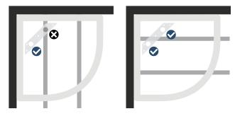
With the unique connect2 design even Quadrant and the Kudos unique Full Curve shape trays have the ability to avoid joists.
